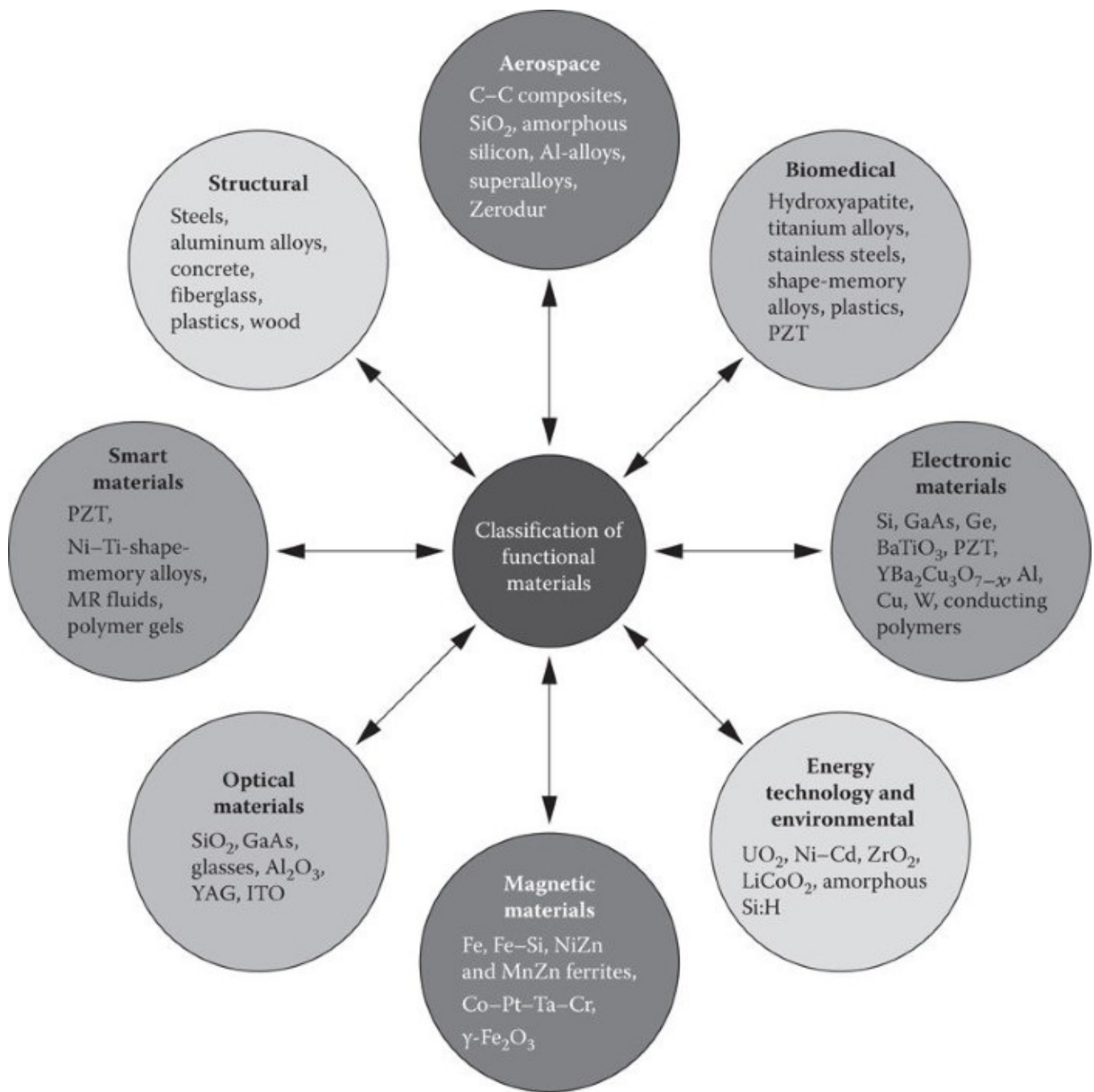
FIGURE 1.8 Functional classification of materials. (From Askeland, D. and Fulay, P., The Science and Engineering of Materials , Thomson, Washington, DC, 2006. With permission.)
